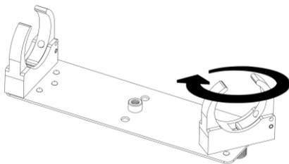
The holders on the Wing Plate can be aligned in parallel if one Wing Plate is used with one tube. In addition, the holders on the Wing Plate can be turned 45° or 90°. That way two tubes can be connected together in different angles.
