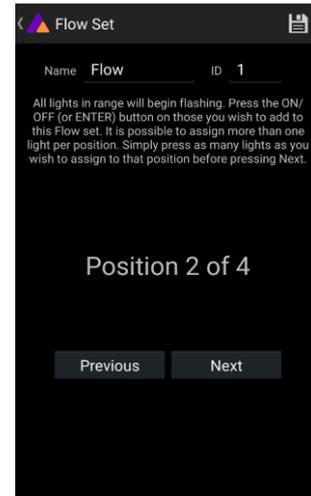
Now your lights will flicker every two seconds. To add a light to the currently shown position of this set, press its button. Walk through the positions by “Previous” and “Next” and assign your lights. When finished, press the save button on top.
