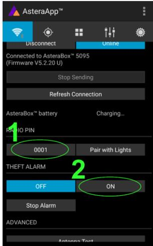
First make sure your Radio PIN is different from 0000. See chapter 8.1 how to change it. Then press the "ON" button.
