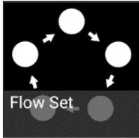
By using a Flow-Set, lights can also be controlled together. But additionally, they are assigned to positions inside the Flow-Set and so form a virtual light with several pixels. All effects, like a running light, are stretched over this virtual light.
