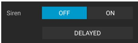
If the siren is set to DELAYED, it sounds only if the alarm persists for more than 6 seconds. The ON setting makes it sound immediately, while the OFF setting mutes it always.
