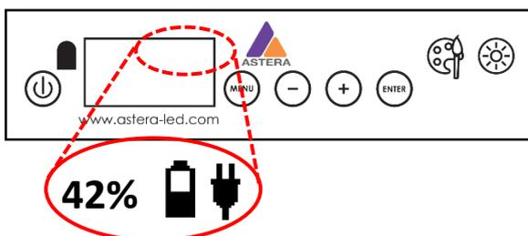
The display at the backside of the Titan Tube contains a battery icon which indicates the rough battery status. Next to it is a percentage that shows a more exact battery status.
